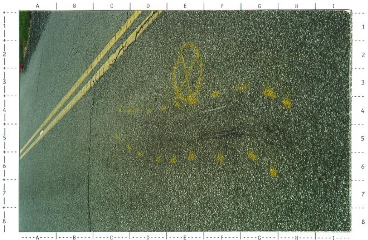
# 28 -- Westward close-up of 1988 Chevrolet pickup's LF skidmark, POI, and point of deflection
